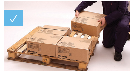
Instruction for non-regular shipment Minimum 4 boxes on pallet Maximum 9 layers of boxes
